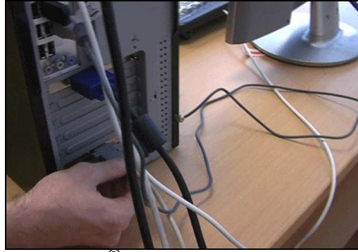
Attaching Wavecom ® DB9 data cable to host serial port
