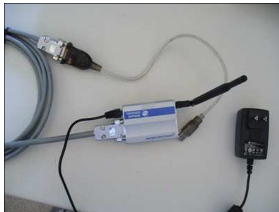
Wavecom Fastrack 20 ® GSM modem kit shown with external antenna and ATEN ® UC232A USB adapter with Wavecom ® 9-15 pin serial data cable.
